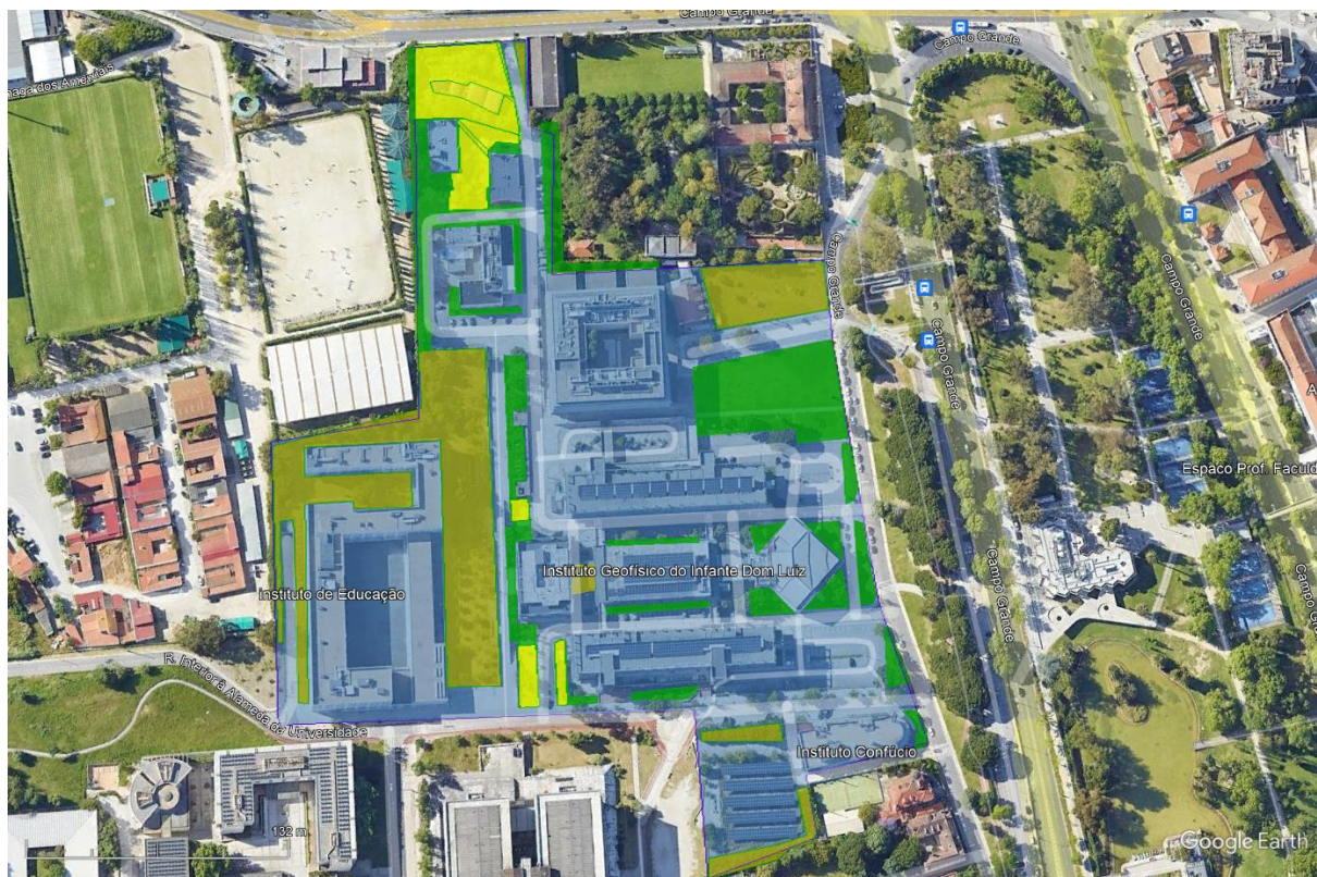
Figure 26 FCUL campus area in Campo Grande, Lisboa. Permeable surfaces (lawns and gardens) are represented in green, while impervious surfaces are highlighted in blue. Brown surfaces (covered with compact sediment) are also featured. HortaFCUL's areas appear in yellow.
