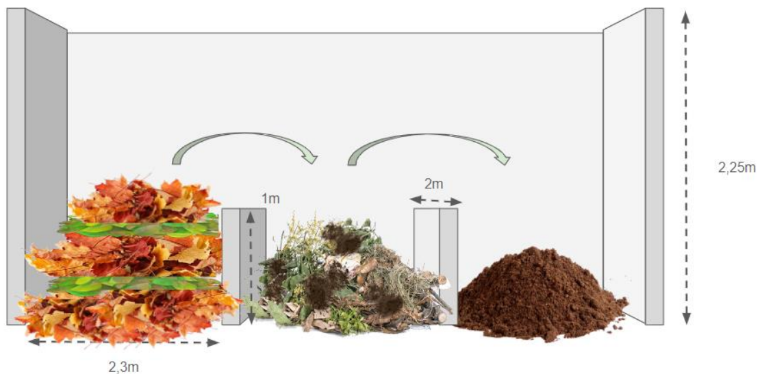
Figure 20 A scheme of HortaFCUL's composting station. Each compartment has an average volume of 4\text{m}^3 . Arrows represent the transfer flux from one compartment to the next to increase the input of oxygen into the pile. Infrastructure is not drawn at scale.
