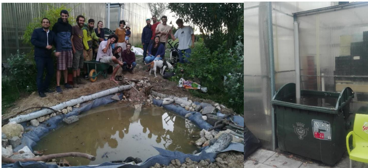
Figure 17 Plant assisted gray water treatment pond (FitoETAR in Portuguese) in PermaLab (left picture) and municipality's obsolete containers used to store stormwater (right picture).
